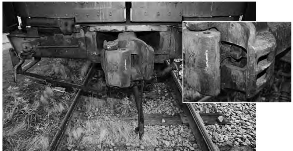
*A defective coupler was at the center of one injured railroad worker case. The coupler is what links each railroad car to the car in front and behind. The coupler’s design is more than 100 years old. It is iron and has four moving parts that don’t always cooperate.*
